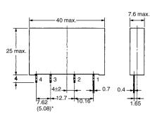
PCB Dimensions (Bottom View) 2.54 Four, 1.2 dia. holes Four, 1.
